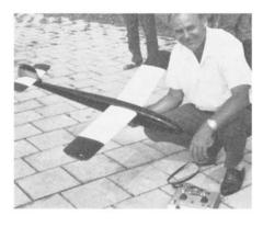
With this small glider Hans Schumacher has set the FAI RC glider speed record at 77.8 mph. It spans 41½" and weighs 44½ oz. This speed bomb is towed aloft by car and then dives to terminal velocity, goes through the speed traps, up and around, and back through once more for both directions.
