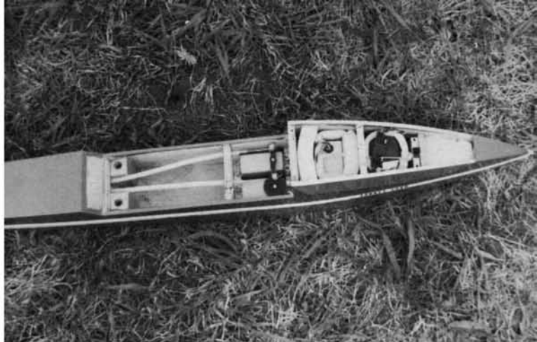
With hatch removed, the servos, Nyrod pushrods, foam-wrapped receiver and battery pack are easily accessible. Radio installation in "Yankee" is easy.
