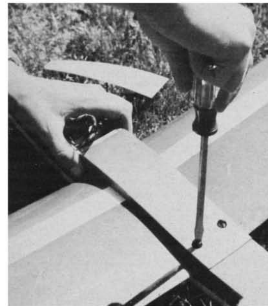
Neil drives down the nylon bolts and all will soon be ready. No grimy rubber bands in sight.
