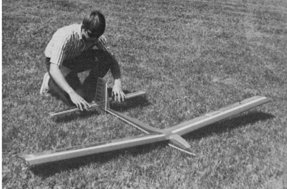
The panels slide home on wire in tubing, standard fare for the giant gliders. Ship ends up compact enough for transport, rugged enough for a winch launch. Wing assumes polyhedral under air load.
