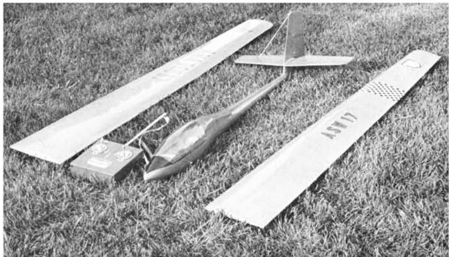
Apart from all that... big as it is, it fits in any car. A fiberglass fuselage, a sheet tail. As on all gliders, nose down for fast response to rudder. Don't overdo it. A capable performer.
